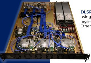
**DLSR2** units perform the analog-to-packets function, using wideband analog-to-digital converters and high-performance FPGAs for signal processing and Ethernet interfaces.
